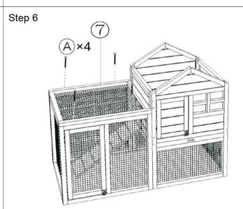
Secure part of using 4x screw(A).
