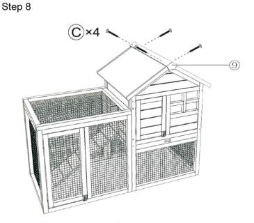
Put on roof cap part 9, secure with 4x screw(C).
