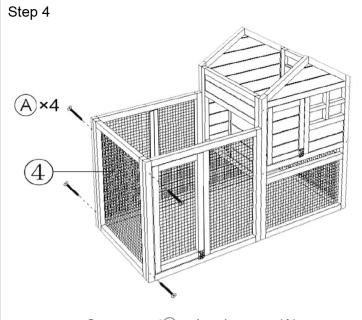
Secure part 4 using 4x screw(A).
