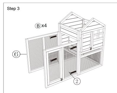
Secure part② and ⑥, each using 2x screw(B) as shown. Note: part② and ⑥ are of the same size.
