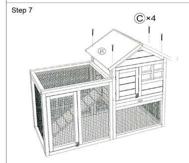
Put on 2x roof part®, each secure with 2x screw(C).
