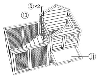
Secure ladder part<sup>①</sup> using 2x screw(D). Then Insert metal tray part<sup>①</sup>
